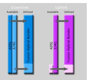
The Fusion Hybrid Bonder uses 80-90% of the ADSI downlink speed and 80-90% of the 3/4G uplink speed to create a hybrid bonded service with the best of both worlds!
